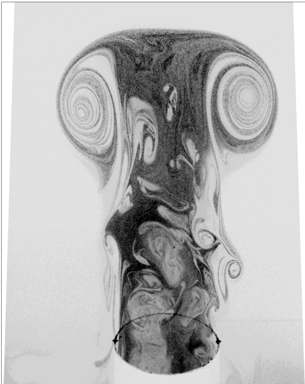
Figure 1. A cross section of a thermal plume generated in a laboratory with use of a humidifier as a buoyancy source. Distribution of condensed water is shown by gray tone (courtesy: Anna Gorska and Szymon Malinowski).
