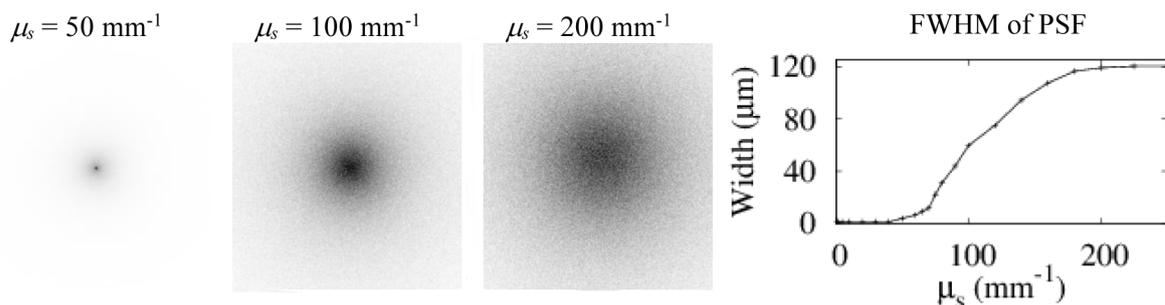
Figure 1: Simulated microscopy images of a point source for various values of  $\mu_s$  (ballistic signal is omitted), and graph of the full width at half maximum of the point spread function as a function of  $\mu_s$ .
