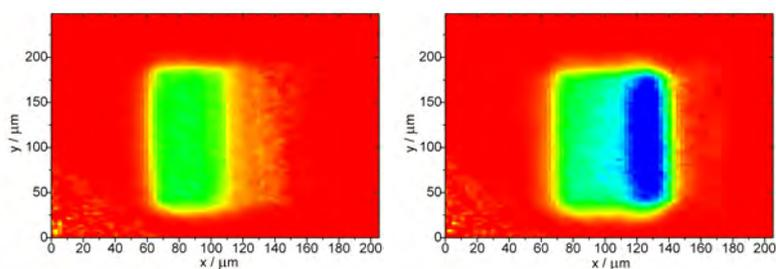
Figure 1: Selected FPA maps of benzene adsorption in a  $175 \mu\text{m} \times 100 \mu\text{m} \times 52 \mu\text{m}$  piece of mesoporous silicon at a pressure of 75 mbar (left map) and 115 mbar (right map) with the 5 nm pores being arranged on the left half and the 10 nm pores on the right half of the sample. Light color represents low, dark color high benzene concentration.
