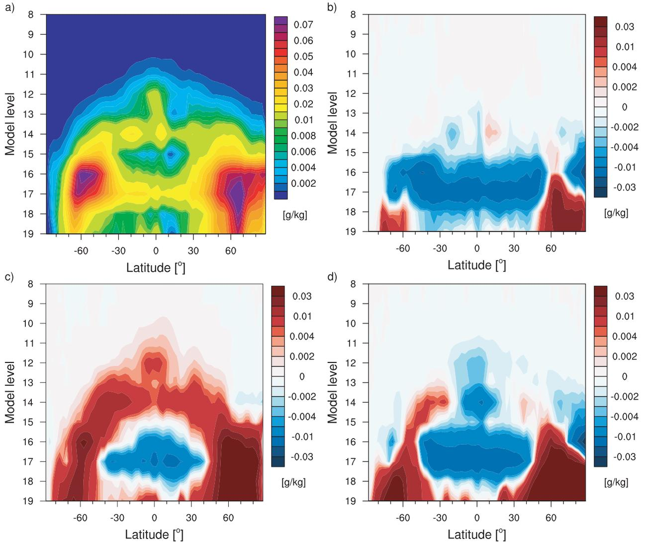
**Figure 3.** (a) Vertical distribution of zonal annual mean cloud liquid water calculated by the original scheme (*orig-b*), (b) untuned version of the new scheme (*rev*) minus the original scheme (*orig-b*), (c) retuned version of the new scheme (*adjust*) minus the original scheme (*orig-b*) and (d) an alternative parameterization (*kk*) minus the original scheme (*orig-b*).
