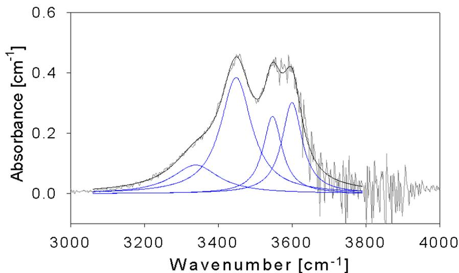
**Fig. 1** IR-spectrum of a fused mullite after water vapor treatment (12 h).
