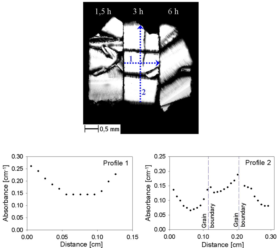
**Fig. 2** Optical micrograph showing the cross sections of fused mullite samples after water vapor treatment (top). The OH-concentration-profiles (bottom) are obtained from the data points measured along the marked lines by means of IR spectroscopy.
