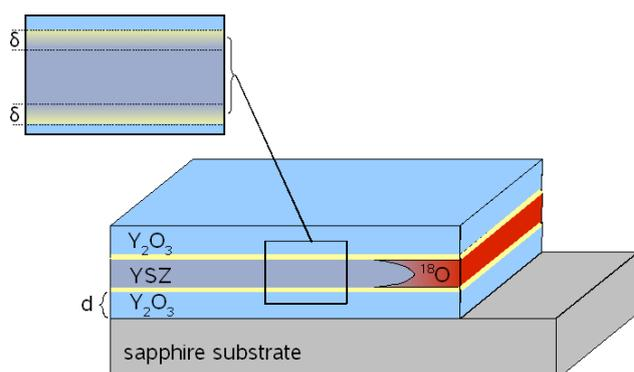
**Fig 1** Schematic illustration of  $^{18}\text{O}$ -tracer diffusion in a  $\text{Y}_2\text{O}_3/\text{YSZ}/\text{Y}_2\text{O}_3$  layer system. The diffusion along the layer interfaces is faster than the bulk diffusion. The layer thickness  $d$  of YSZ and  $\text{Y}_2\text{O}_3$  is the same.  $\delta$  is assigned to the region between the layers of the ion conductor and insulator which corresponds to the interface.
