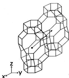
Fig. 1: Schematic view of the chabazite framework.
