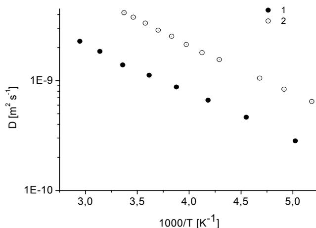
Fig. 1: **Temperature dependence of effective diffusion coefficient** 1 – diffusion coefficient in glass bed of sample 3; 2 – diffusion coefficient of pure liquid n-hexane
