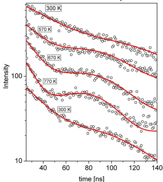
Fig. 1: The NRS time spectra of the Fe monolayer on W(110) registered at temperatures 300, 570, 670, 700, 300 K. For clarity, the spectra are shifted relatively to each other.
