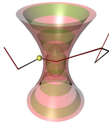
Fig. 1: PhoCS working principle – a colloidal particle enters the focal domain, is heated and the resulting change in solvent index of refraction is detected.
