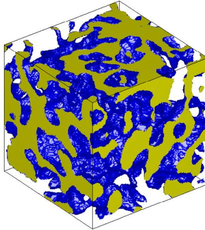
Fig. 1. 3D stochastic replica shown as a subregion of  $160 \times 160 \times 160$  voxels. Pore orifices are yellow, pore-solid interface is blue, and solid matrix is transparent.
