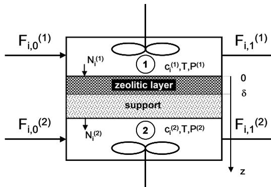
Fig. 1: Scheme of W-K cell
