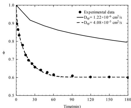
Fig. 1: Concentration decay curve of pyridine on CAG predicted with the pore volume diffusion model.
