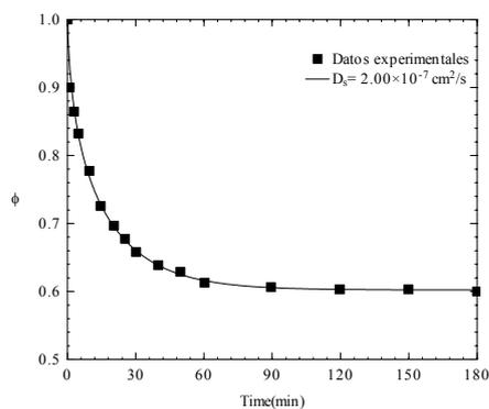
Fig. 2: Concentration decay curve of pyridine on CAG predicted with the superface diffusion model.
