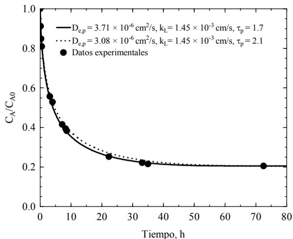
Fig. 1: Concentration decay curves for fluoride adsorption on GBC. The lines represent the diffusional model predictions. Run No. 2.
