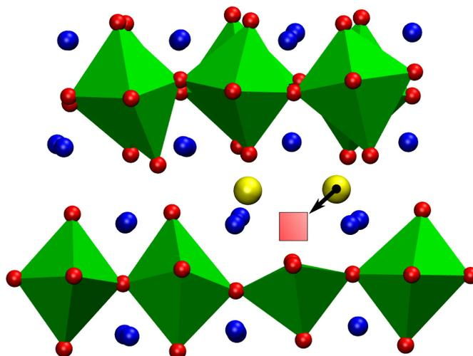
Fig. 1: The observed oxygen interstitialcy mechanism in  $\text{La}_2\text{NiO}_{4+\delta}$  [4].
