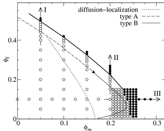
Fig. 1: Kinetic diagram of the HS QA system. White circles: equilibrated. Black circles: glassy. Thin lines: MCT transition lines [3]. Thick line: arrest line from simulations, defined via  $\delta r^2(t)$ .
