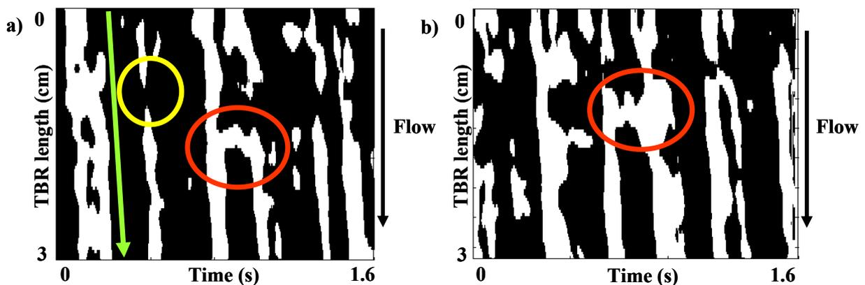
Figure 2: MR images showing the splitting and merging of liquid pulses as they travel down the bed at  $L = 0.011 \text{ ms}^{-1}$ ,  $G = 0.36 \text{ ms}^{-1}$  at 3.3 bar. The liquid pulses appear white and gas pulses black. Indicated in the red circles: (a) splitting of one liquid pulse (b) merging of part of a liquid pulse with another. The gradient of the green line corresponds to the average fluid (gas + liquid) velocity.
