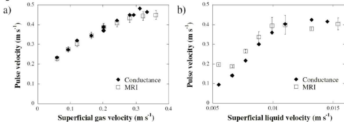
Figure 1: Pulse velocity calculated from both conductance and MRI techniques. (a) As a function of the gas flow rate when  $L = 0.011 \text{ ms}^{-1}$ . (b) As a function of the liquid flow rate when  $G = 0.20 \text{ ms}^{-1}$  at 3.3 bar. The error bars are the standard deviation of the results obtained in different experiments.
