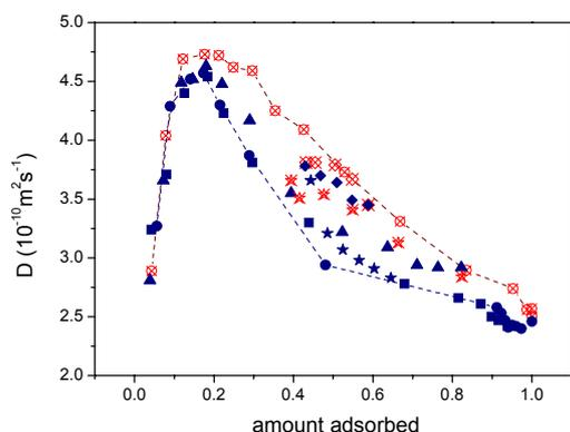
**Fig. 3.** The diffusivities from Fig. 2b plotted versus the relative amount adsorbed using the data of Fig. 2a. Also diffusivities obtained more complex cycles of the pressure variation are shown.
