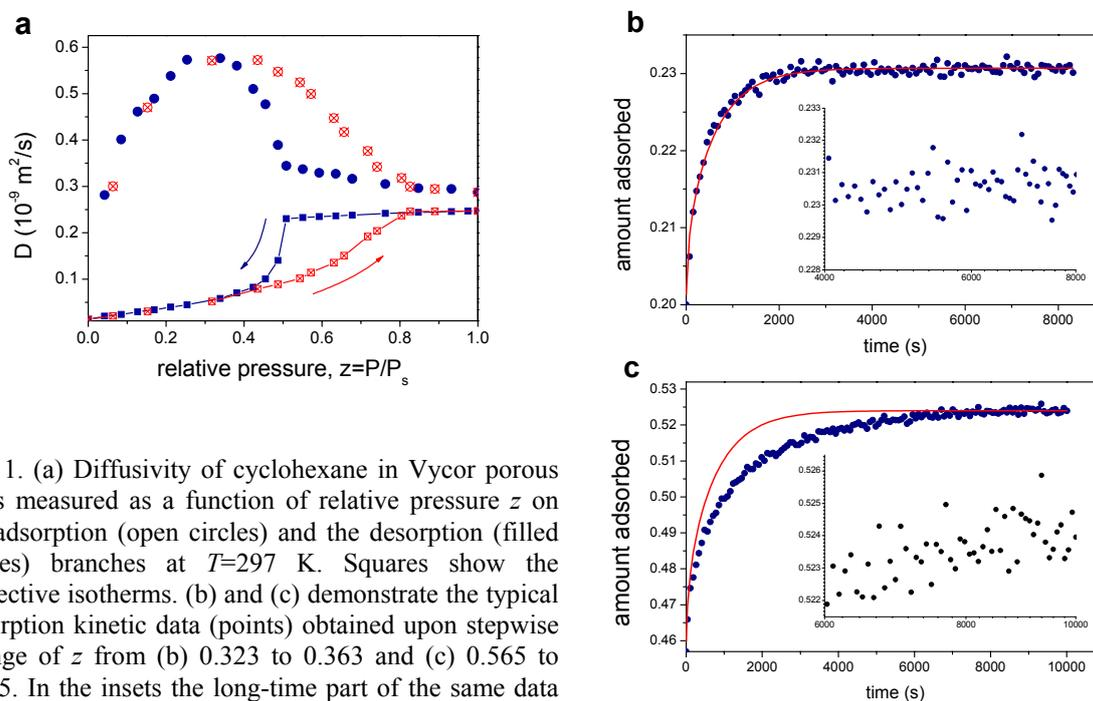
Fig. 1. (a) Diffusivity of cyclohexane in Vycor porous glass measured as a function of relative pressure  $z$  on the adsorption (open circles) and the desorption (filled circles) branches at  $T=297$  K. Squares show the respective isotherms. (b) and (c) demonstrate the typical adsorption kinetic data (points) obtained upon stepwise change of  $z$  from (b) 0.323 to 0.363 and (c) 0.565 to 0.605. In the insets the long-time part of the same data are shown.
