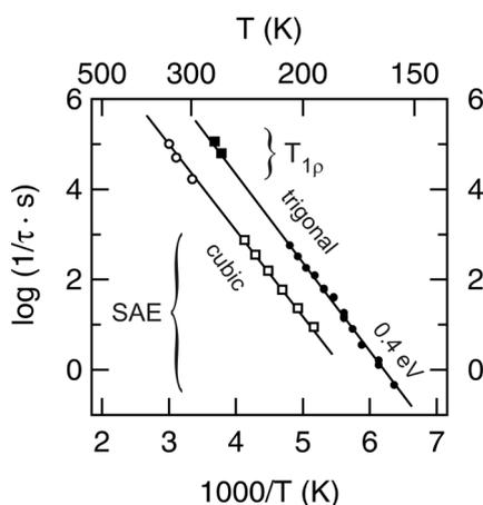
Fig. 1: Arrhenius plot of slow Li jump rates in cubic Li<sub>0.6</sub>TiS<sub>2</sub> and trigonal Li<sub>0.7</sub>TiS<sub>2</sub>. In both cases the Li transport process is thermally activated with  $\approx 0.4$  eV.
