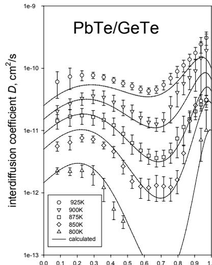
Fig. 1: Interdiffusion coefficient for GeTe/PbTe alloys
