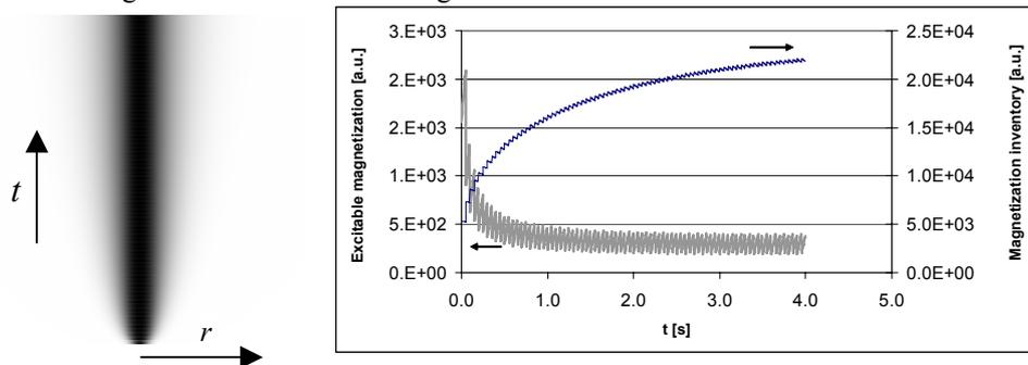
Fig. 1: Left side: Simulation of the spatiotemporal spreading of excited magnetization (grayshades) from a 30  $\mu\text{m}$  slice of water ( $T_1$  3 s) under the action of periodic 90° pulses applied every 50 ms. Right side: Development of the amount of excitable in-slice magnetization and the overall inventory of excited nuclear magnetization present in the sample.
