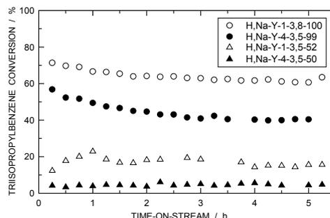
**Figure 2:** Catalytic conversion of 1,3,5-triisopropylbenzene over zeolite H,Na-Y.
