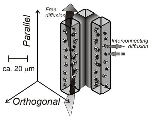
**Figure 1.** Principal structure of tracheid cells. The two anisotropic self-diffusion paths are shown.
