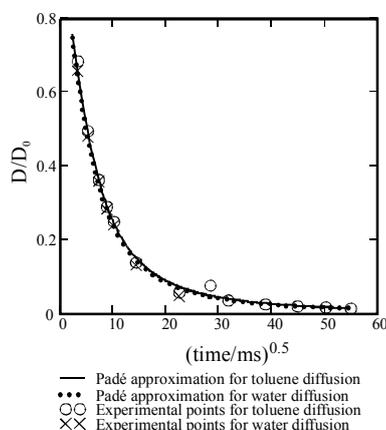
**Figure 2.** Experimental diffusion coefficients of toluene and water in sapwood. The lines are fits to Padé-approximants.
