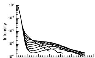
Figure 1. Stejskal Tanner plots from water in a gel emulsion. The gradient pulse length is varied from 1.5 to 50 ms. under conditions of constant gradient pulse area.
