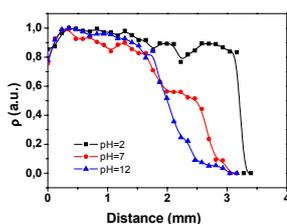
Fig.1. The spin-density  $\rho$  profiles of solvent protons within the gel layer of HPMC
