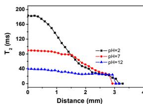
Fig.2. The spin-spin  $T_2$  profiles of solvent protons within the gel layer of HPMC
