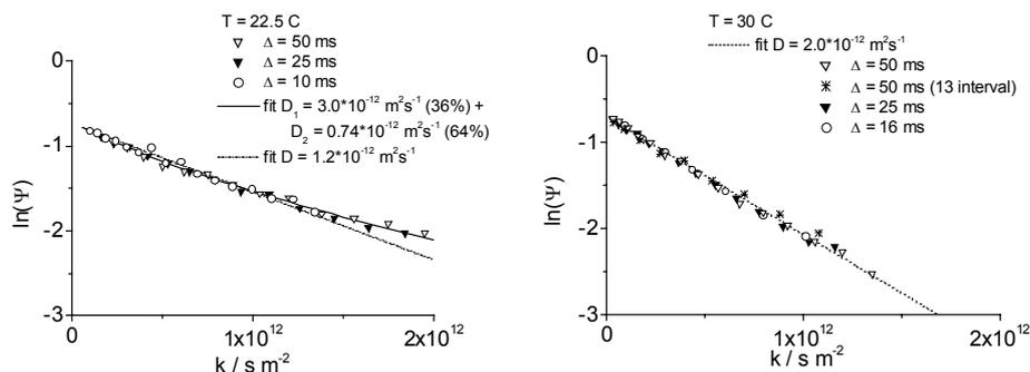
**Fig. 1:**  $^1\text{H}$  PFG NMR attenuation curves measured for two different temperatures. The figure on the left (right) side shows the data points including a two-exponential (one-exponential) fit.
