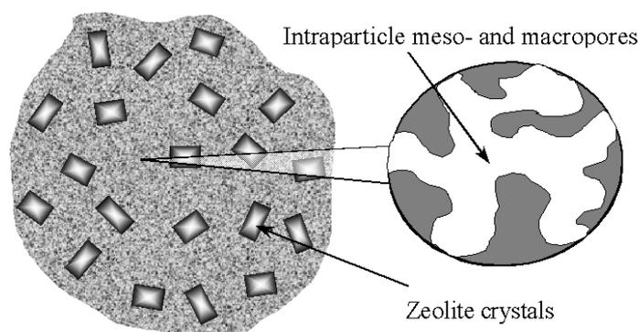
Fig.1 Schematic presentation of a particle of a typical FCC catalyst.
