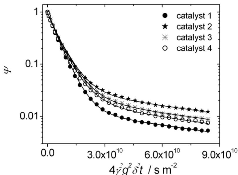
Fig.2 <sup>1</sup>H PFG NMR spin echo attenuation curves (points) measured by using the 13-interval PFG NMR sequence for 1,3,5 tri-iso-propyl-benzene in different FCC catalysts containing the same fraction of the same zeolite USY. The diffusion time in all cases was equal to 30 ms. Lines show the best fit of the experimental curves by using Eq.3 with  $N=3$ . The best fit parameters are presented in Table 1.
