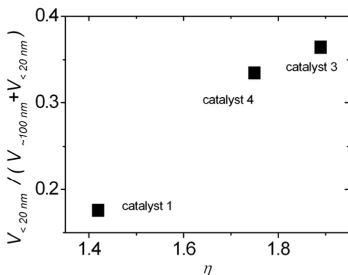
Fig.3 Correlation between the fraction of the intraparticle meso- and macropores with sizes smaller than 20 nm and the tortuosity factors for diffusion of 1,3,5 tri-iso-propyl-benzene in the intraparticle pores
