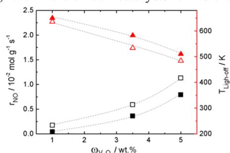
Figure 2: Reaction rate ( $r_{\text{NO}}$ ) at 523 K and light-off temperature ( $T_{\text{Light-off}}$ ) during SCR-DeNO<sub>x</sub> over mesoporous and hierarchical V<sub>2</sub>O<sub>5</sub>/TiO<sub>2</sub> catalysts with different V<sub>2</sub>O<sub>5</sub>-content.
