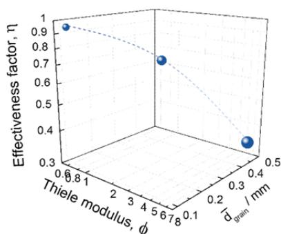
Figure 1: Effectiveness factor and Thiele modulus for different grain sizes of the 5 wt.% V<sub>2</sub>O<sub>5</sub>/TiO<sub>2</sub> mesoporous catalyst.
