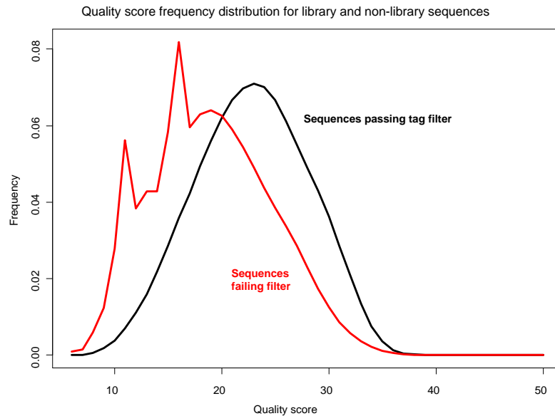
Figure 3.12: Sequences resulting from crystals, dust and lint particles as well as other flow cell features are typically of low complexity (figure 3.11 on the preceding page) but only partially of low quality. Plotted is the quality score frequency distribution (PHRED-scale [63], Ibis base caller [116]) for all reads matching the 'GAC' library tag in the beginning of the read (black, n = 557,466,159 bases from 10,930,709 reads) as well as all sequences not matching the tag sequence and its one base pair substitutions (red, n = 3,481,668 bases from 68,268 reads). The data was obtained from lane 5 of the 080902_BIOLAB29_Run_PE51.1 run from the Neandertal Genome project [81].
