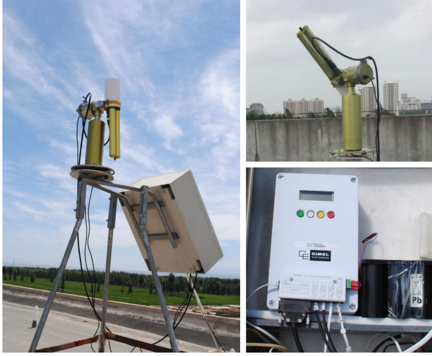
Figure 3.1: The new ground-based CIMEL Dual-Polar sun/sky radiometer (left: CE318-DP#962; top-right: the optical sensor head fixed on the automated mount; bottom-right: the electronic box ).
