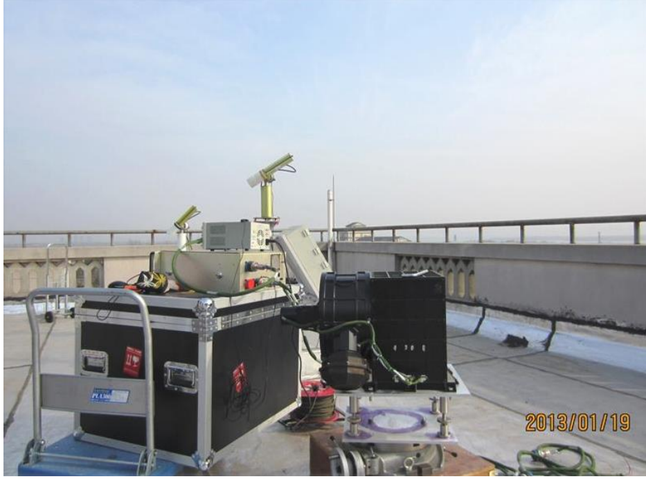
Figure 5.4: Ground-based synchronous observations by the CE318-DP #962 and the AMPR on 19 January, 2013 in Hefei, China (31.9N, 117.2E).
