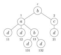
As shown in above diagram, the positions in pos(t) describe the "path" we have to take from the root in order to get to the according node in the graph. The subtree  $t|_{13}$  of t at position 13 is:
